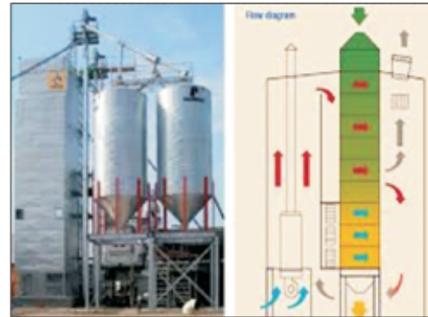
Continuous flow dryer
